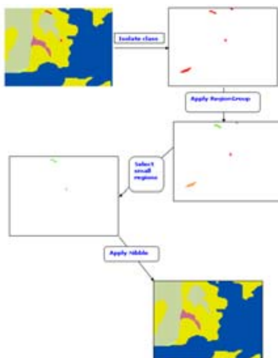
Figure 82. Steps for removal of noisy pixels
