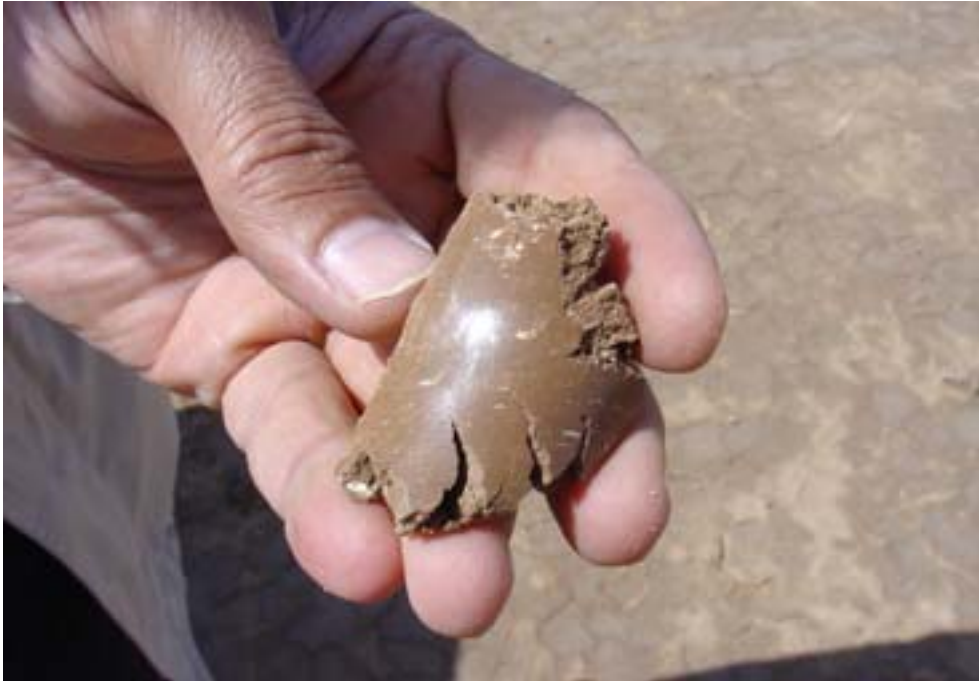
Figure 63. The prevalence of clayey soils developed on fine alluvium makes drainage and leaching of salts difficult.
