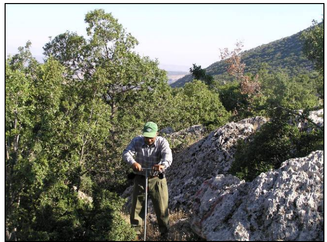
Fig. 5 Measurements of soil depth /cm
